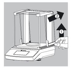
B) Remove the top glass cover:1) Holding it by its rear edge, pull the draft shield cover up.2) Remove the draft shield cover.
