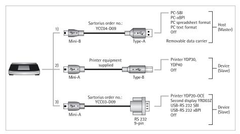
There are three ways to connect the balance via USB:
