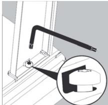
6) Turn the key approx. two times to loosen the Torx screws.
