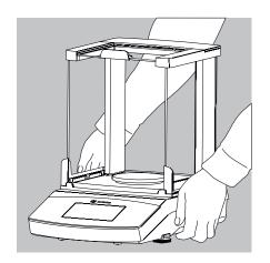
▶ Hold the balance under the housing, lift it up carefully, and carry it to its new location.
