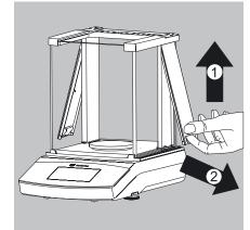
Remove the Torx key up from the draft shield under the cover.
