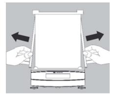
7) Pull out the draft shield frame from the side of the guide
