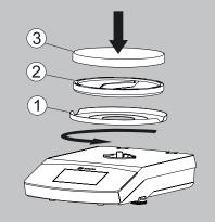
3) Install the pan support (2) and weighing pan (3).
