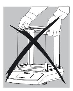
Avoid glass breakage, shocks, and vibrations: Never lift or carry the balance when holding it by its draft shield!
